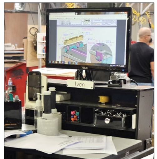
Left —Nine Fusion XL CNC machines from Komo (each running 12 different cutter heads and 20 drill bits) are the heart of production at Teak Isle. Right —Each of the thousands of parts it produces has a complex computer file with part history, design specifications, materials, hardware and assembly details, and cutting parameters for the router.
