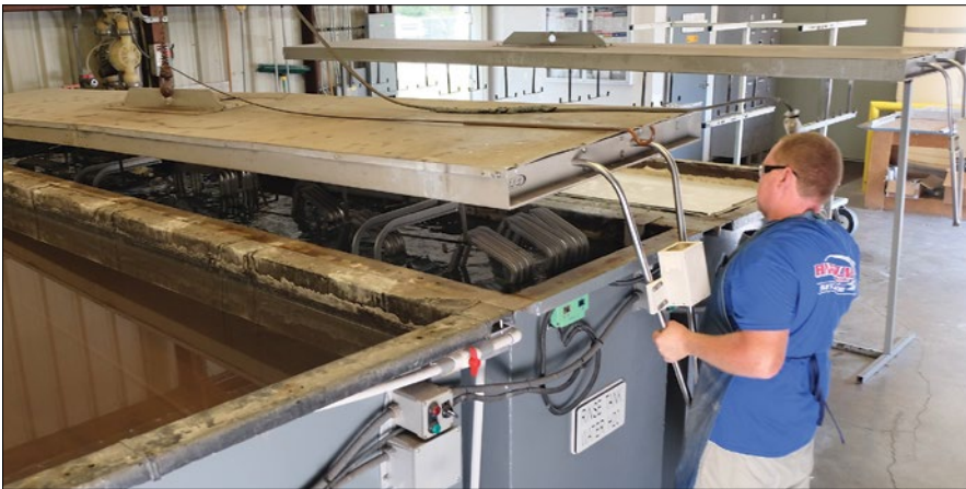
Above left —In the metal shop, CNC bending machines form extruded aluminum stock into custom frames. Left —In preparation for finish powder-coating, frames are run through a series of chemical baths and distilled-water rinses. Above —Racks of drilling fixtures for specific frames in the metal shop. These guides ensure that the manually drilled holes for installation and mounting hardware perfectly correspond to those in the plastic panels they marry to.
