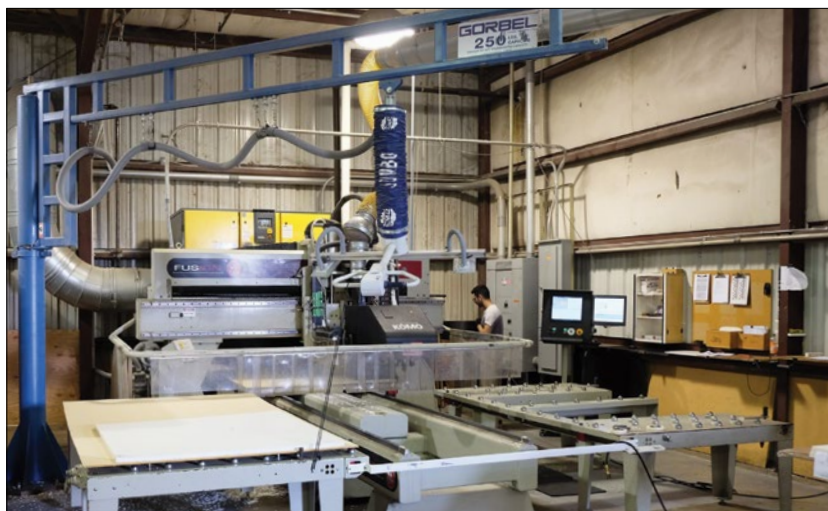
Left —Nine Fusion XL CNC machines from Komo (each running 12 different cutter heads and 20 drill bits) are the heart of production at Teak Isle. Right —Each of the thousands of parts it produces has a complex computer file with part history, design specifications, materials, hardware and assembly details, and cutting parameters for the router.
