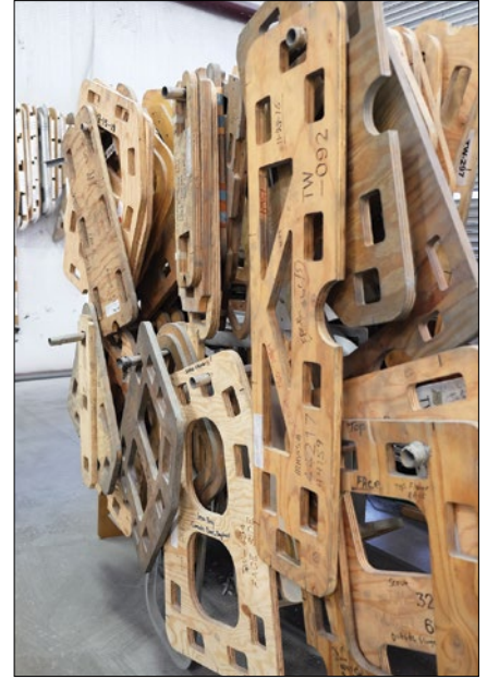
Above left —In the metal shop, CNC bending machines form extruded aluminum stock into custom frames. Left —In preparation for finish powder-coating, frames are run through a series of chemical baths and distilled-water rinses. Above —Racks of drilling fixtures for specific frames in the metal shop. These guides ensure that the manually drilled holes for installation and mounting hardware perfectly correspond to those in the plastic panels they marry to.
